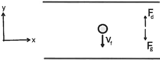
Figure 4: Mechanical equilibrium without an \vec{E} field gives rise to a falling terminal velocity \vec{v}_f , as the only two forces are drag ( \vec{F}_d ) and gravity ( \vec{F}_g ).
